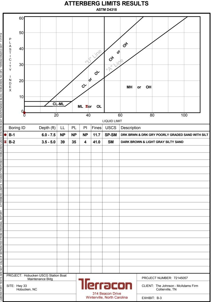
ATTERBERG LIMITS 72145057 PROPOSED HOBUCKEN USCG STATION BOAT MAINTENANCE BLDG; HOBUCKEN, NC. GPJ TERRACON2012. GDT 11/17/14 -ABORATORY TESTS ARE NOT VALID IF SEPARATED FROM ORIGINAL REPORT. APPENDIX C SUPPORTING DOCUMENTS
